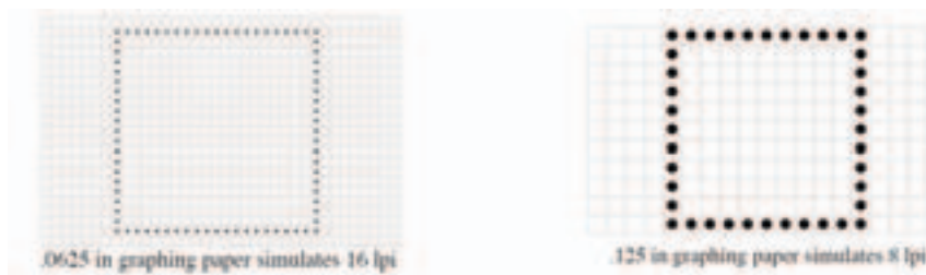
Figure 6. When a viewer can no longer distinguish 16 LPI dots, 8 LPI dots can still be discerned.
