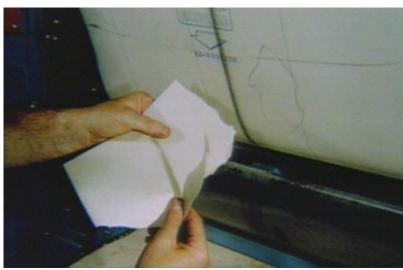
It is worth repeating that a careful packing of the plate and blanket cylinders is important for quality printing. A single thousandth error in packing will mean the difference between a high quality and a poor job.
