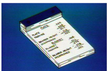
(4) Installing plate and blanket with packing sheets;
