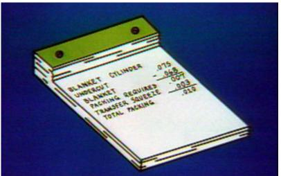
...second, to accurately adjust the plate-toblanket pressure necessary for ink transfer;
