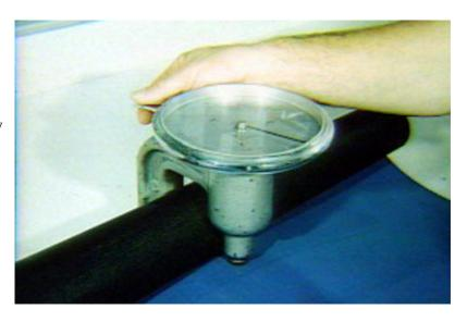
The *Blanket Thickness Gauge*, developed by GATF, is a specially designed bench micrometer with a large throat that allows for easy measurement at any point on the blanket surface.
