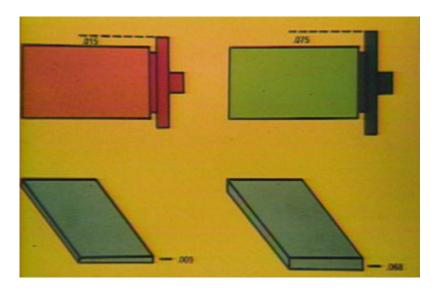
For example, if the undercut for the blanket cylinder is .075" and the blanket is .068", the packing required to bring the blanket to bearer height would be .007".
