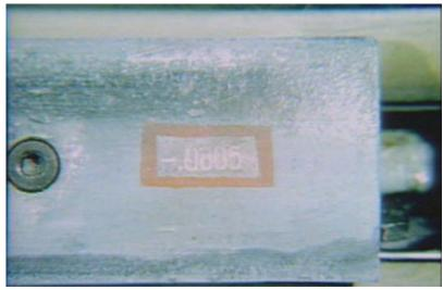
Then, plate and blanket are carefully "miked." A machinist's micrometer can be used to mike the thickness of the plate and packing sheets. Although relatively easy to use, care must be taken to get an accurate reading.
