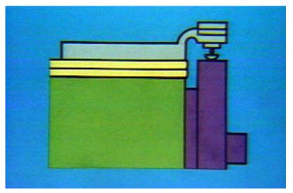
The surface height of a newly installed blanket should be rechecked occasionally with the packing gauge until the blanket and packing have settled. Although the cylinders may have originally packed properly, packing sheets may compress under the transfer-squeeze pressure. After a short amount of running, this compression results in an underpacked condition.
