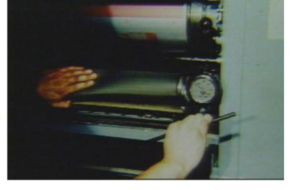
Special care must be taken when tightening the plate firmly around the plate cylinder. Excessive tension on the plate may crack the plate at the clamps. Only tighten the plate until it is firmly held against the cylinder body and packing. Check this by tapping
