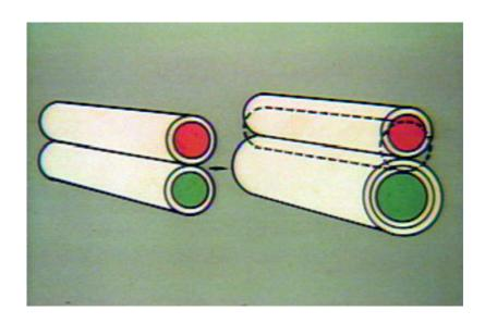
Cylinder diameters are changed for several reasons: first, to allow for varying thicknesses of plates and blankets;
