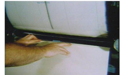
Square the packing sheets with the plate or blanket and place them to overlap the leading edge of the cylinders so that they will not slip while running.
