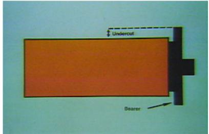
The amount of undercut must be known in order to calculate the amount of packing required to bring the plate of blanket up to bearer height.
