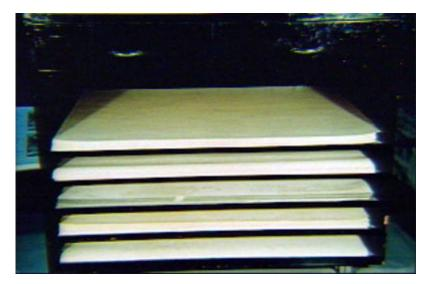
For convenience, pre-cut packing sheets, identified by distinctive colors for each thickness, should be stored near each press. The color coding helps in selecting packing sheets when a press is to be made ready.
