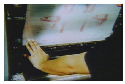
The blanket must be carefully and securely fastened onto the blanket bars before being mounted onto the cylinder where it has to be held perfectly square and parallel to the cylinder.
