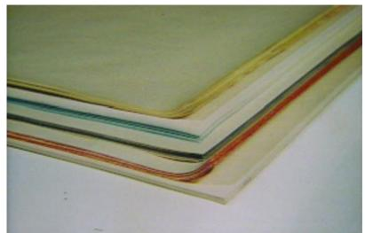
When determining the amount of sheets required for packing, a press operator should keep the number of packing sheets used under the plate and blanket to a minimum.
