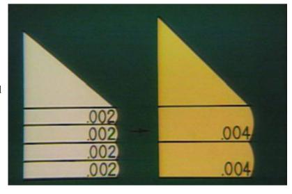
Packing sheets for the blanket cylinder should be cut slightly narrower than the blanket. The packing sheets for the plate cylinder are cut the same width as the plate.
