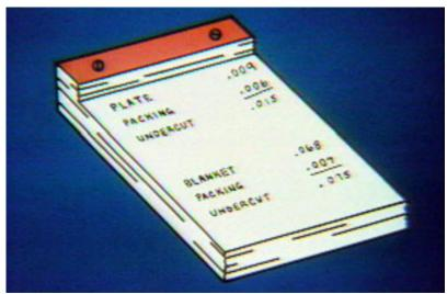
Accurate packing of plate and blanket cylinders is essential for good presswork, especially with the popular use of fine-grained or grainless plates, A difference of .001" may seriously affect the quality of printing or reduce the life of plates.
