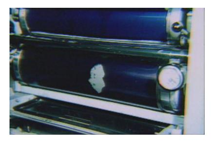
To determine whether the low spot is in the blanket or the cylinder body, clean and remove the blanket; then turn it so that the trailing edge will now become the lead edge. If the low spot is in the blanket, it will appear again in the same area of the blanket surface when the press is put on impression again. If it remains in the same area in relation to the cylinder body, then the low spot may be in the body of either the plate or blanket cylinder.
