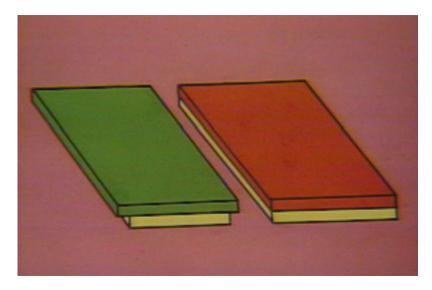
Presses that "run on bearers" have plate and blanket cylinder bodies that are cut below the bearer surface. The difference between the surface of the bearers and the surface of the cylinder body is called the **undercut**.
