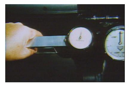
The "local" type of packing is termed *patching*. This is done with tissue to make up for local depressions in the blanket or the cylinders.
