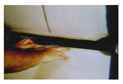
(5) Checking accuracy of measurements and calculations with the packing gauge; and (6) Rechecking after running a short time.
