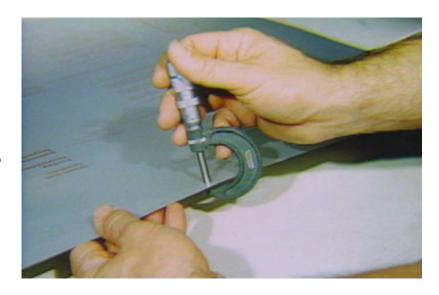
Machinist's micrometers are not suitable for measuring blanket thickness because the small anvil and spindle surfaces will compress the soft blanket.
