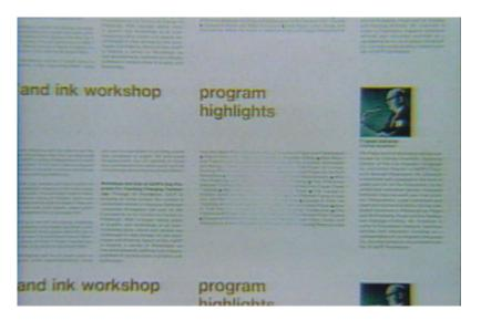
Low spots can be easily located by completely inking a gummed plate and running the press on impression. Low areas will appear as clear or slightly inked in the solid print on the blanket.
