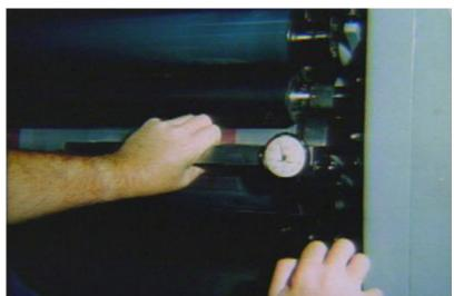
The packing gauge is an instrument designed to measure the height of the plate or blanket in relation to the bearer height after they have been mounted on the cylinders with proper packing.
