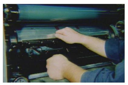
Finally, after the cylinders are packed and the blanket and plate are tight, the height of the packed cylinders is checked with a packing gauge.
