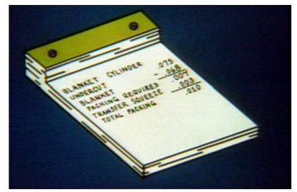
It is essential that you check with the manufacturer's instructions as to how the plate and blanket cylinders should be packed for a particular press. Mike the plates and blankets with their packing to determine the actual thickness.
