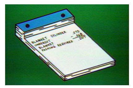
Calculations for the plate cylinder packing is done in the same manner. The undercut for the plate cylinder is less than the undercut of the blanket cylinder because plates are thinner than blankets.
