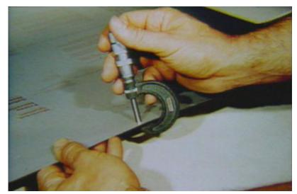
(3) Calculating the amount of packing necessary to bring plate and blanket to proper height;
