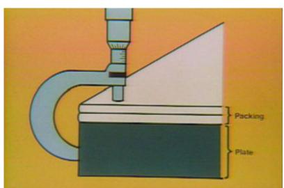
Fourth, install the blanket and then the plate. Plates with positioning marks must be carefully lined up with the corresponding plate cylinder marks.
