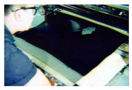
Using the bulge as a guide, outline the low area by drawing on the back of the blanket. This will give the exact size and location for the patch which will be applied to the back of the blanket.
