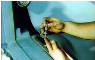
Micrometers with larger anvil and spindle surfaces--such as paper micrometers--are more accurate, but their small throats limit measurement only to the blanket edges.
